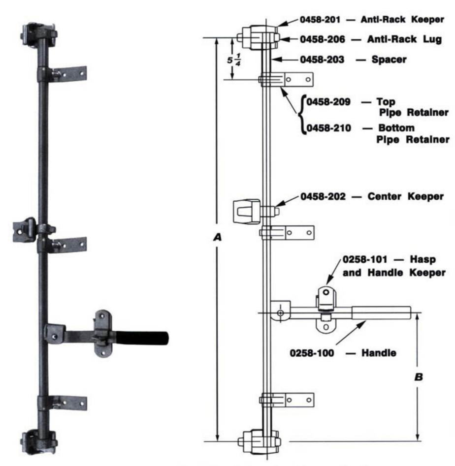
No. 458-008 Two Point Anti-Rack Lock (less pipe)
